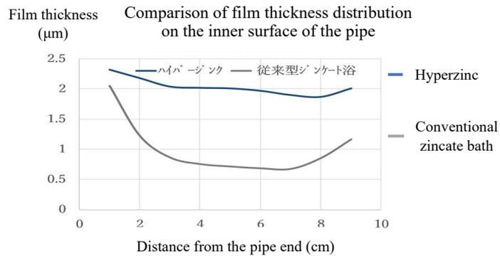
Figure 2: Comparison of plating throwing power of low current parts
