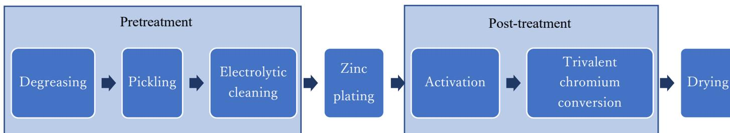
Figure 4: Zinc plating process (general processing process)
