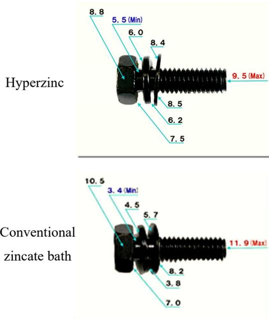
Figure 1: Comparison of film thickness distribution (barrel plating)
